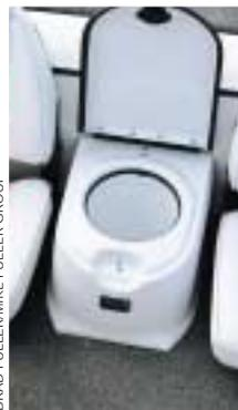
Fore and aft decks offering more than 56 square feet of fishing room are just the start of this boat's angling amenities. (Far left) Our test boat's helm features wheel-mounted trim switches, SmartCraft gauges and a flush-mount Garmin sounder. The custom gearshift works well and looks great. (Left) The trash compartment/emergency head hinges up to reveal a 5-gallon pail. The entire assembly tilts forward for access to livewell pumps.
