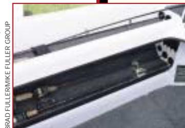
Gunwale rod lockers to port and starboard feature disappearing, sliding doors. Running rod racks above each locker have tubes to protect rod tips from elephant-footed friends.
