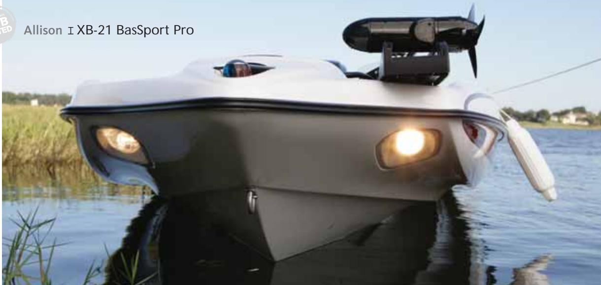
**Docking lights are standard with the BasSport Pro. They're recessed under the unique Allison hull, behind clear Lexan lenses. Optional driving lights are set behind the same set of lenses.**
